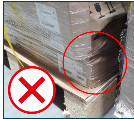
Apply edge protection over entire pallet height (and width) – not only partially.
