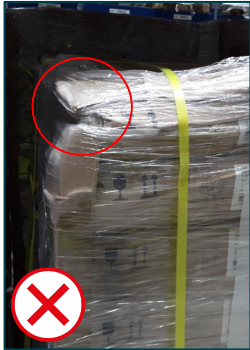
Apply edge protection over entire pallet height (and width) – not only partially.
