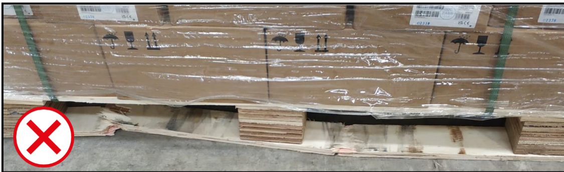
Insufficient quality, poor processing (e.g. pallet feet glued from single wooden plates or chipboard)
