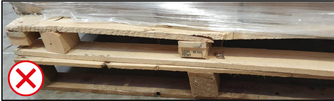
Insufficient quality, poor processing
