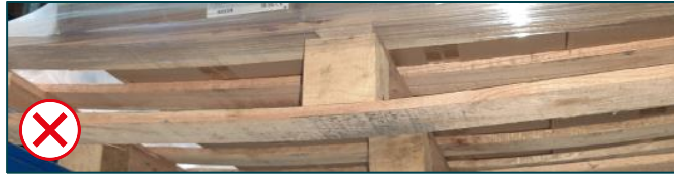
Load too heavy: pallet bends
