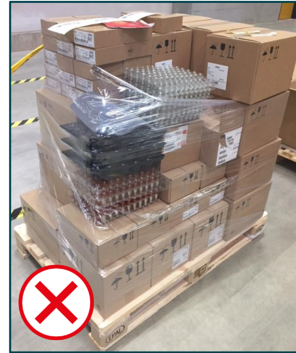
No loose goods on the pallet, all goods must be packed in carton.
